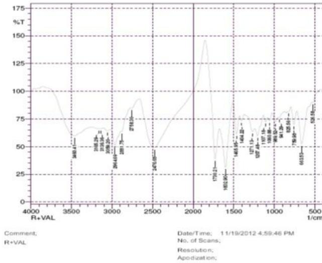
**Fig.6** FTIR spectra of Mannitol
