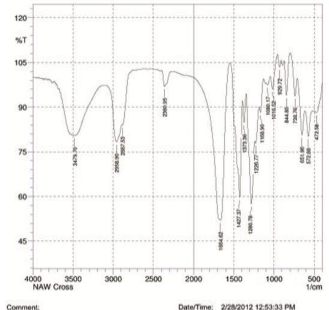
**Fig.9 FTIR spectra of VAL: Mannitol (1:4) KM**
