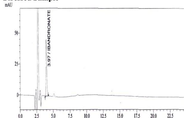
Figure.7 Overlaid Chromatogram of Heat Stressed Sample
